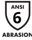
**ABRASION ANSI 6** offer a superior durability. Level **6/6** mean the glove can resist till more than 20 000 cycles of 180 grits abrasive material before perforated the glove.
